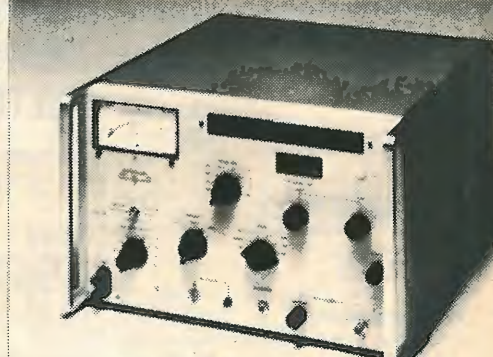
HEWLETT PACKARD WAVE ANALYSER TYPE 310A 1kHz - 1.5MHz. 10µV - 100V. Dynamic range 75dB. B.F.O. and recorder O/P. Built in AM, LSB & USB Detector. £1,200.00
