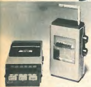
GENERAL RADIO SOUND LEVEL METER 1933 WITH CASSETTE DATA RECORDER 1935 & C weighting. 10dB-130dB. Equipped with 1/2 microphone. Wide band analyser with 10 octave freqs. 31.5Hz-16KHz. Uses high quality C60 cassettes. Fully operated. £2,600.00
